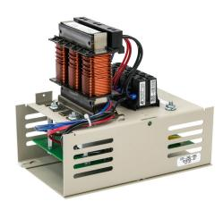
AutomationDirect VTF series drive output filter, 208-600 VAC, 3hp at 208/230 VAC, 7-1/2hp at 460 VAC and 10hp at 575 VAC, 3-phase, 12A, output side only. For use with multiple AC drives.
