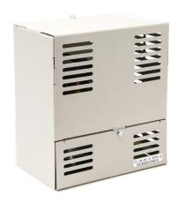
AutomationDirect VTF series drive output filter, 208-600 VAC, 3hp at 208/230 VAC, 7-1/2hp at 460 VAC and 10hp at 575 VAC, UL Type 1, 3-phase, 12A, output side only. For use with multiple AC drives.
