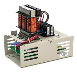
AutomationDirect VTF series drive output filter, 208-600 VAC, 2hp at 208/230 VAC and 5hp at 460/575 VAC, 3-phase, 8A, output side only. For use with multiple AC drives.
