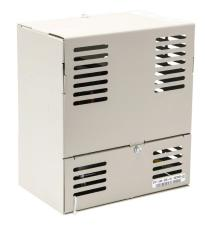
AutomationDirect VTF series drive output filter, 208-600 VAC, 1/2hp at 208/230 VAC, 1-1/2hp at 460 VAC and 2hp at 575 VAC, UL Type 1, 3-phase, 3A, output side only. For use with multiple AC drives.
