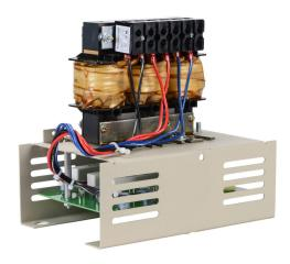
AutomationDirect VTF series drive output filter, 208-600 VAC, 5hp at 230 VAC and 10hp at 460 VAC, 3-phase, 16A, output side only. For use with multiple AC drives.
