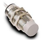
Micro Detectors inductive proximity sensor, tubular, 30mm diameter x 60mm body, nickel-plated brass housing, N.O. output, 15mm sensing distance, non-flush, 25 Hz switching frequency, IP67, pigtail.
