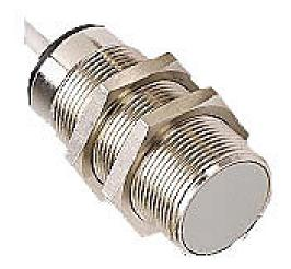
Micro Detectors inductive proximity sensor, tubular, 30mm diameter x 60mm body, nickel-plated brass housing, N.O. output, 10mm sensing distance, flush, 25 Hz switching frequency, IP67, pigtail.
