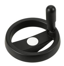
Elesa handwheel, spoked, 125mm diameter, 12mm bore, foldaway revolving handle, polypropylene, matte black.
