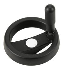
Elesa handwheel, spoked, 4in diameter, 3/8in bore, foldaway revolving handle, polypropylene, matte black.
