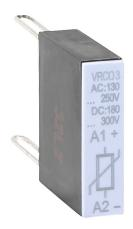
WEG Electric surge suppressor, varistor, 130-275 VAC/180-300 VDC. For use with CWC07 through CWC025 series miniature contactor.
