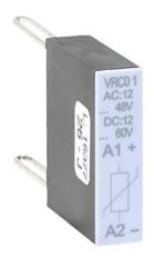
WEG Electric surge suppressor, varistor, 12-48 VAC/12-60 VDC. For use with CWC07 through CWC025 series miniature contactor.
