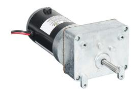
IronHorse VP1 series parallel shaft DC gear motor, 1/25hp, 90 VDC, 94rpm, 13 lb-in full load torque, 0.31 FLA, 26:1 ratio, 5/16in shaft diameter.
