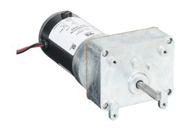
IronHorse VP1 series parallel shaft DC gear motor, 1/25hp, 90 VDC, 29rpm, 40 lb-in full load torque, 0.31 FLA, 83.5:1 ratio, 5/16in shaft diameter.
