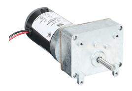
IronHorse VP1 series parallel shaft DC gear motor, 1/50hp, 90 VDC, 11rpm, 50 lb-in full load torque, 0.19 FLA, 269:1 ratio, 5/16in shaft diameter.
