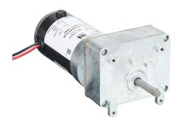
IronHorse VP1 series parallel shaft DC gear motor, 1/50hp, 90 VDC, 7rpm, 50 lb-in full load torque, 0.15 FLA, 386:1 ratio, 5/16in shaft diameter.
