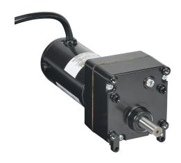
IronHorse VP1 series parallel shaft DC gear motor, 1/11hp, 90 VDC, 139rpm, 42 lb-in full load torque, 1.19 FLA, 24:1 ratio, 1/2in shaft diameter.
