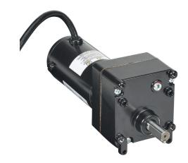
IronHorse VP1 series parallel shaft DC gear motor, 1/11hp, 90 VDC, 71rpm, 83 lb-in full load torque, 1.29 FLA, 52:1 ratio, 1/2in shaft diameter.
