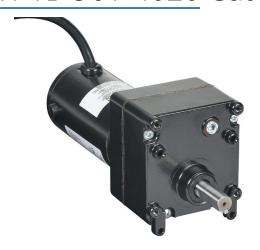
IronHorse VP1 series parallel shaft DC gear motor, 1/17hp, 90 VDC, 20rpm, 100 lb-in full load torque, 0.5 FLA, 102:1 ratio, 1/2in shaft diameter.
