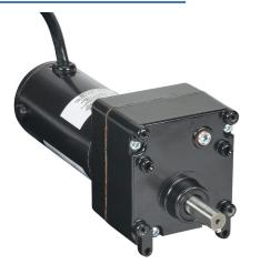
IronHorse VP1 series parallel shaft DC gear motor, 1/25hp, 90 VDC, 139rpm, 20 lb-in full load torque, 0.63 FLA, 16:1 ratio, 1/2in shaft diameter.
