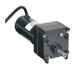
IronHorse VP1 series parallel shaft DC gear motor, 1/25hp, 90 VDC, 37rpm, 74 lb-in full load torque, 0.67 FLA, 79:1 ratio, 1/2in shaft diameter.
