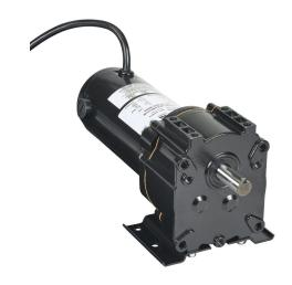
IronHorse VP1 series parallel shaft DC gear motor, 1/4hp, 90 VDC, 83rpm, 160 lb-in full load torque, 2.53 FLA, 30:1 ratio, 5/8in shaft diameter.
