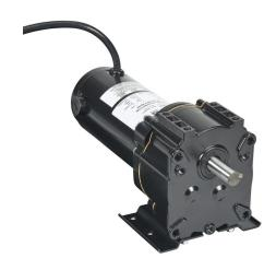
IronHorse VP1 series parallel shaft DC gear motor, 1/4hp, 90 VDC, 42rpm, 280 lb-in full load torque, 2.45 FLA, 57.7:1 ratio, 5/8in shaft diameter.
