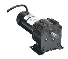
IronHorse VP1 series parallel shaft DC gear motor, 1/8hp, 90 VDC, 165rpm, 47 lb-in full load torque, 1.57 FLA, 11:1 ratio, 5/8in shaft diameter.
