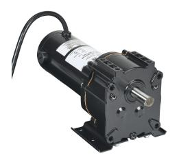
IronHorse VP1 series parallel shaft DC gear motor, 1/8hp, 90 VDC, 91rpm, 86 lb-in full load torque, 1.58 FLA, 20:1 ratio, 5/8in shaft diameter.
