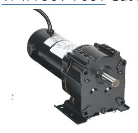
IronHorse VP1 series parallel shaft DC gear motor, 1/8hp, 90 VDC, 61rpm, 113 lb-in full load torque, 1.42 FLA, 30:1 ratio, 5/8in shaft diameter.
