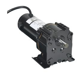
IronHorse VP1 series parallel shaft DC gear motor, 1/8hp, 90 VDC, 54rpm, 138 lb-in full load torque, 1.51 FLA, 34:1 ratio, 5/8in shaft diameter.
