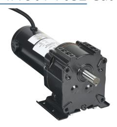
IronHorse VP1 series parallel shaft DC gear motor, 1/8hp, 90 VDC, 32rpm, 220 lb-in full load torque, 1.5 FLA, 58:1 ratio, 5/8in shaft diameter.
