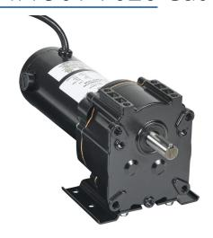
IronHorse VP1 series parallel shaft DC gear motor, 1/8hp, 90 VDC, 26rpm, 280 lb-in full load torque, 1.58 FLA, 69:1 ratio, 5/8in shaft diameter.
