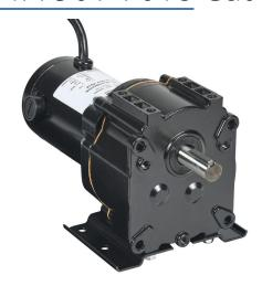
IronHorse VP1 series parallel shaft DC gear motor, 1/8hp, 90 VDC, 18rpm, 150 lb-in full load torque, 0.82 FLA, 103:1 ratio, 5/8in shaft diameter.
