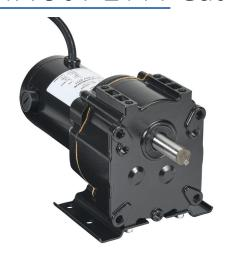
IronHorse VP1 series parallel shaft DC gear motor, 1/20hp, 90 VDC, 111rpm, 28 lb-in full load torque, 0.97 FLA, 17.5:1 ratio, 5/8in shaft diameter.
