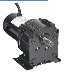
IronHorse VP1 series parallel shaft DC gear motor, 1/20hp, 90 VDC, 51rpm, 55 lb-in full load torque, 0.94 FLA, 34:1 ratio, 5/8in shaft diameter.
