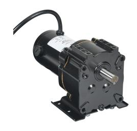
IronHorse VP1 series parallel shaft DC gear motor, 1/20hp, 90 VDC, 34rpm, 82 lb-in full load torque, 0.94 FLA, 57.7:1 ratio, 5/8in shaft diameter.
