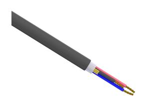
Southwire control cable, unshielded, 3 conductors, 18 AWG, bare copper, PVC/Nylon conductor insulation material, method 1 table 2 color code, PVC jacket, black, cut to length.
