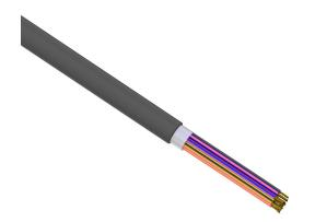
Southwire control cable, unshielded, 19 conductors, 18 AWG, bare copper, PVC/Nylon conductor insulation material, method 1 table 2 color code, PVC jacket, black, cut to length.
