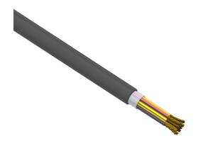
Southwire control cable, unshielded, 12 conductors, 18 AWG, bare copper, PVC/Nylon conductor insulation material, method 1 table 2 color code, PVC jacket, black, cut to length.
