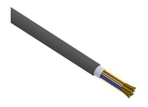
Southwire control cable, unshielded, 10 conductors, 18 AWG, bare copper, PVC/Nylon conductor insulation material, method 1 table 2 color code, PVC jacket, black, cut to length.
