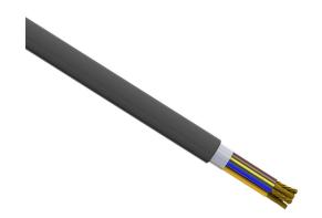
Southwire control cable, unshielded, 9 conductors, 16 AWG, bare copper, PVC/Nylon conductor insulation material, method 1 table 2 color code, PVC jacket, black, cut to length.
