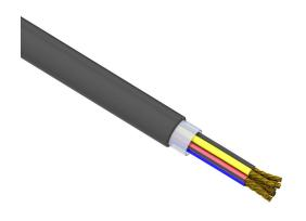
Southwire control cable, unshielded, 7 conductors, 16 AWG, bare copper, PVC/Nylon conductor insulation material, method 1 table 2 color code, PVC jacket, black, cut to length.
