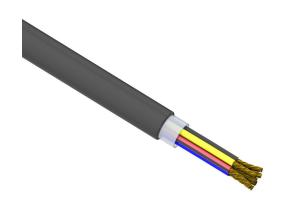
Southwire control cable, unshielded, 7 conductors, 16 AWG, bare copper, PVC/Nylon conductor insulation material, method 1 table 2 color code, PVC jacket, black, cut to length.
