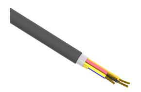
Southwire control cable, unshielded, 5 conductors, 16 AWG, bare copper, PVC/Nylon conductor insulation material, method 1 table 2 color code, PVC jacket, black, cut to length.
