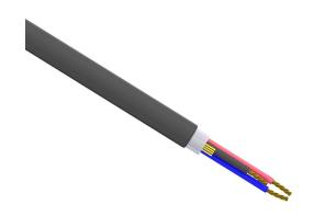
Southwire control cable, unshielded, 3 conductors, 16 AWG, bare copper, PVC/Nylon conductor insulation material, method 1 table 2 color code, PVC jacket, black, cut to length.
