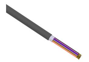
Southwire control cable, unshielded, 19 conductors, 16 AWG, bare copper, PVC/Nylon conductor insulation material, method 1 table 2 color code, PVC jacket, black, cut to length.
