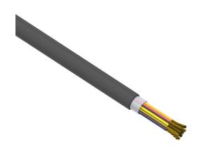
Southwire control cable, unshielded, 12 conductors, 16 AWG, bare copper, PVC/Nylon conductor insulation material, method 1 table 2 color code, PVC jacket, black, cut to length.
