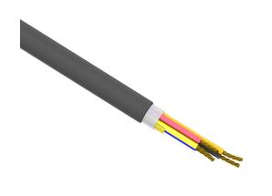
Southwire control cable, unshielded, 5 conductors, 14 AWG, bare copper, PVC/Nylon conductor insulation material, method 1 table 2 color code, PVC jacket, black, cut to length.
