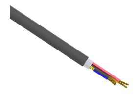
Southwire control cable, unshielded, 4 conductors, 14 AWG, bare copper, PVC/Nylon conductor insulation material, method 1 table 2 color code, PVC jacket, black, cut to length.
