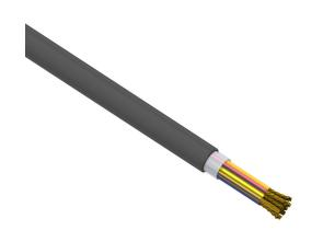
Southwire control cable, unshielded, 12 conductors, 14 AWG, bare copper, PVC/Nylon conductor insulation material, method 1 table 2 color code, PVC jacket, black, cut to length.
