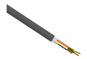
Southwire control cable, unshielded, 5 conductors, 12 AWG, bare copper, PVC/Nylon conductor insulation material, method 1 table 2 color code, PVC jacket, black, cut to length.
