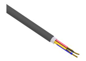
Southwire control cable, unshielded, 4 conductors, 12 AWG, bare copper, PVC/Nylon conductor insulation material, method 1 table 2 color code, PVC jacket, black, cut to length.
