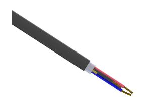
Southwire control cable, unshielded, 3 conductors, 12 AWG, bare copper, PVC/Nylon conductor insulation material, method 1 table 2 color code, PVC jacket, black, cut to length.
