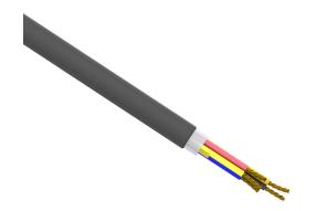
Southwire control cable, unshielded, 5 conductors, 10 AWG, bare copper, PVC/Nylon conductor insulation material, method 1 table 2 color code, PVC jacket, black, cut to length.
