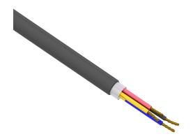
Southwire control cable, unshielded, 4 conductors, 10 AWG, bare copper, PVC/Nylon conductor insulation material, method 1 table 2 color code, PVC jacket, black, cut to length.
