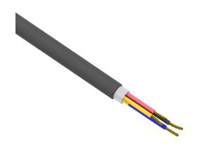
Southwire control cable, unshielded, 4 conductors, 10 AWG, bare copper, PVC/Nylon conductor insulation material, method 1 table 2 color code, PVC jacket, black, cut to length.
